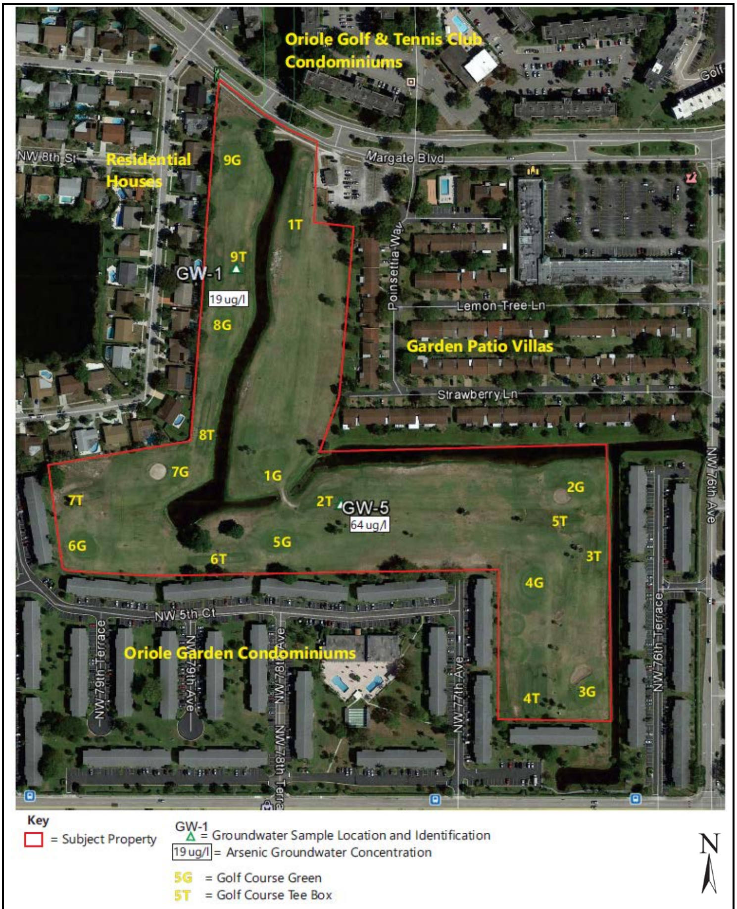
FIGURE 4: SITE PLAN SHOWING GROUNDWATER CONCENTRATIONS Project No. 18-206246.1
