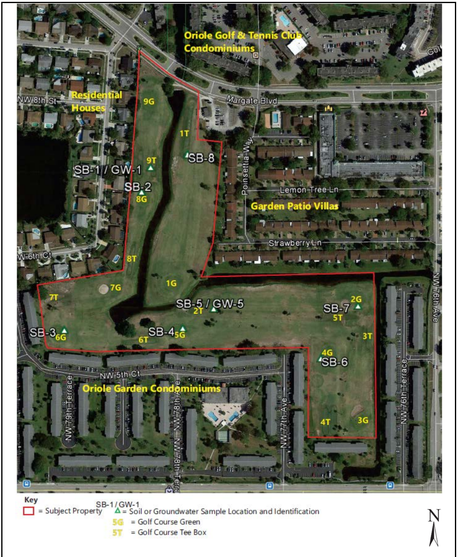
FIGURE 3: SITE PLAN SHOWING SAMPLE LOCATIONS Project No. 18-206246.1
