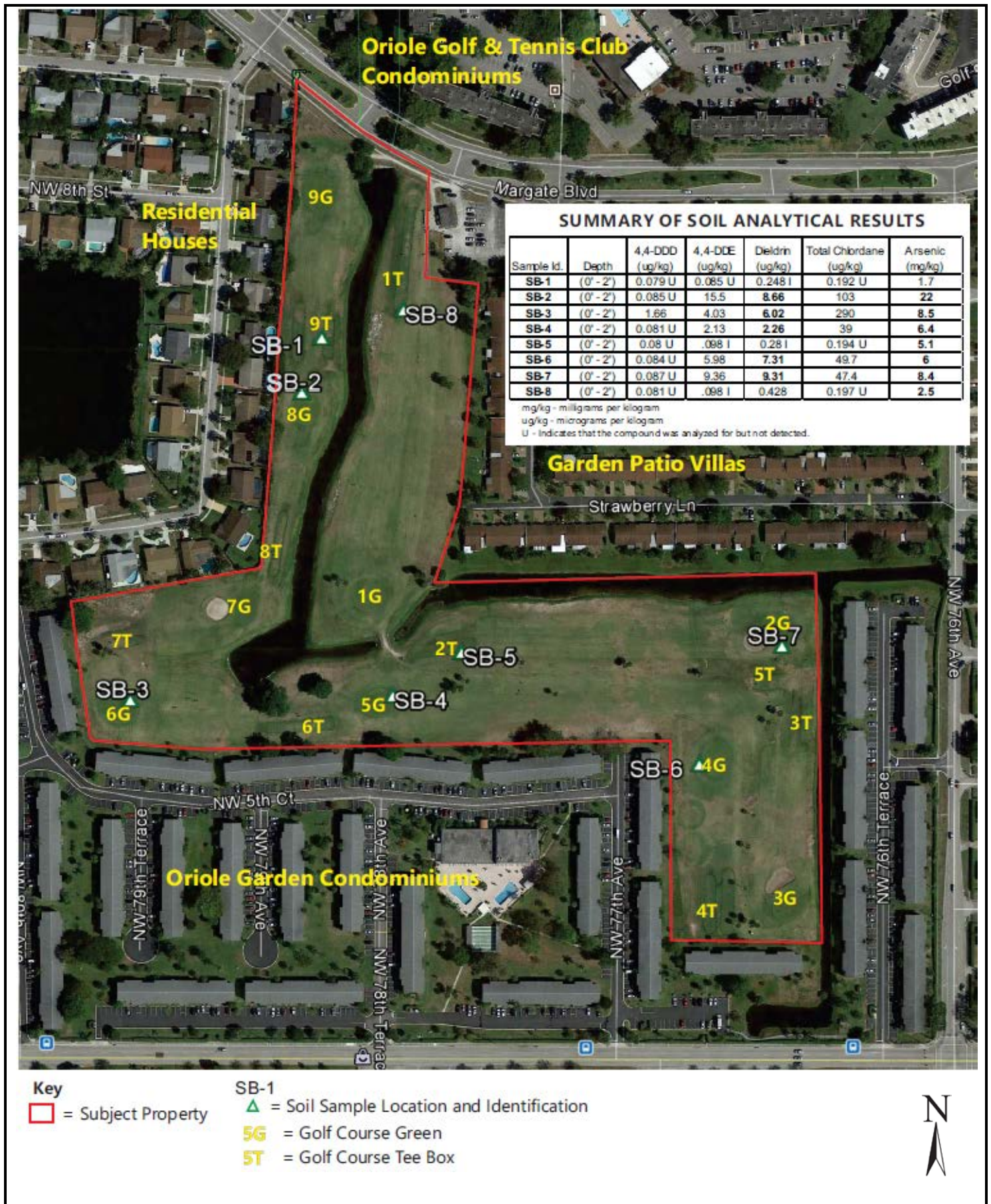
FIGURE 4: SITE PLAN SHOWING SOIL CONCENTRATIONS Project No. 18-206246.1
