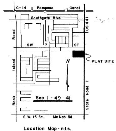
@ P.R.M. - indicates Permanent Reference Monument B.M. - indicates Bench Mark ++++++ - indicates Non- Vehicular Access Line This plat contains 16.0957 acres Coordinates and bearings, as shown, refer to Transverse Mercator Grid System, Florida East Zone, per Misc. P.B. 4, P. 21, B.C.R. This plat is restricted to: 146,000 sq.ft. of office
