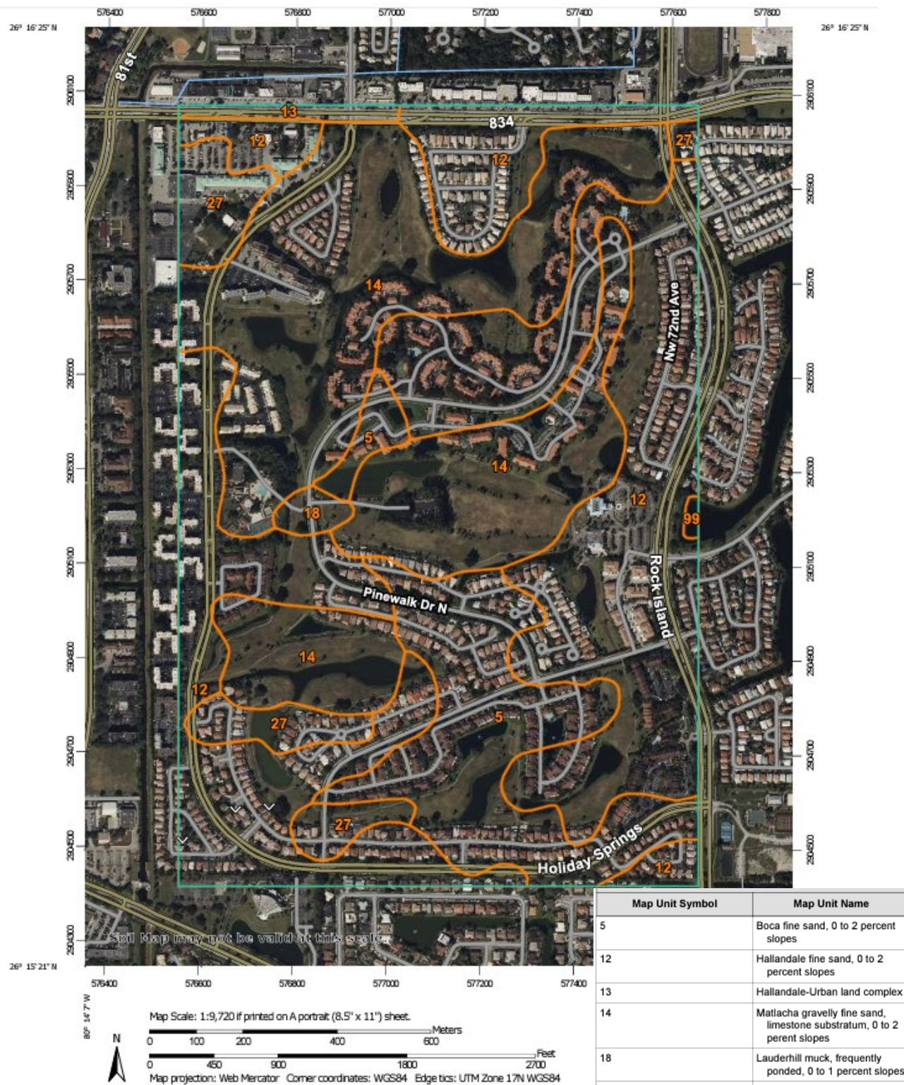
Figure 3. Soil Map (source: NRCS web soil survey)
