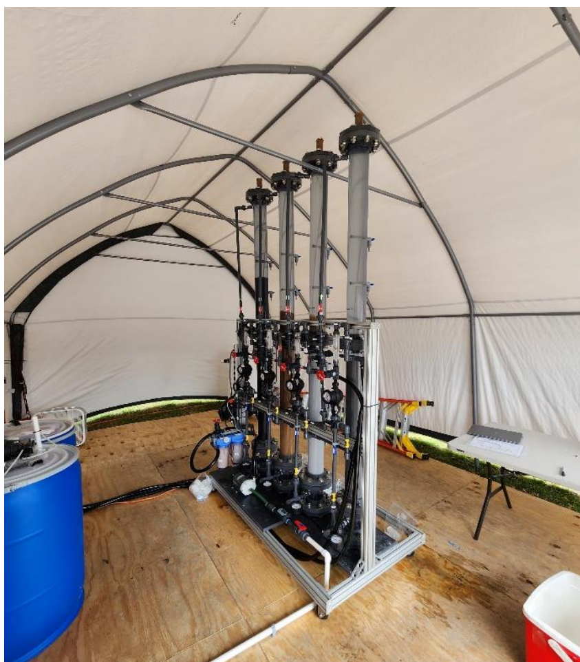
Figure 3-5: City of Margate Ion Exchange Pilot Skid
