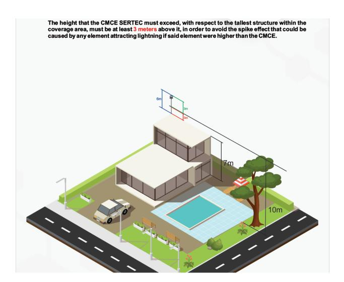
The fixing of the CMCE can vary according to the type of structure to which it must be fixed or according to the internal requirements of the industry. But in each case, it must be guaranteed that this fixing is the safest possible capable of supporting the weight of the equipment plus the mast and winds of up to 150 km/h.
