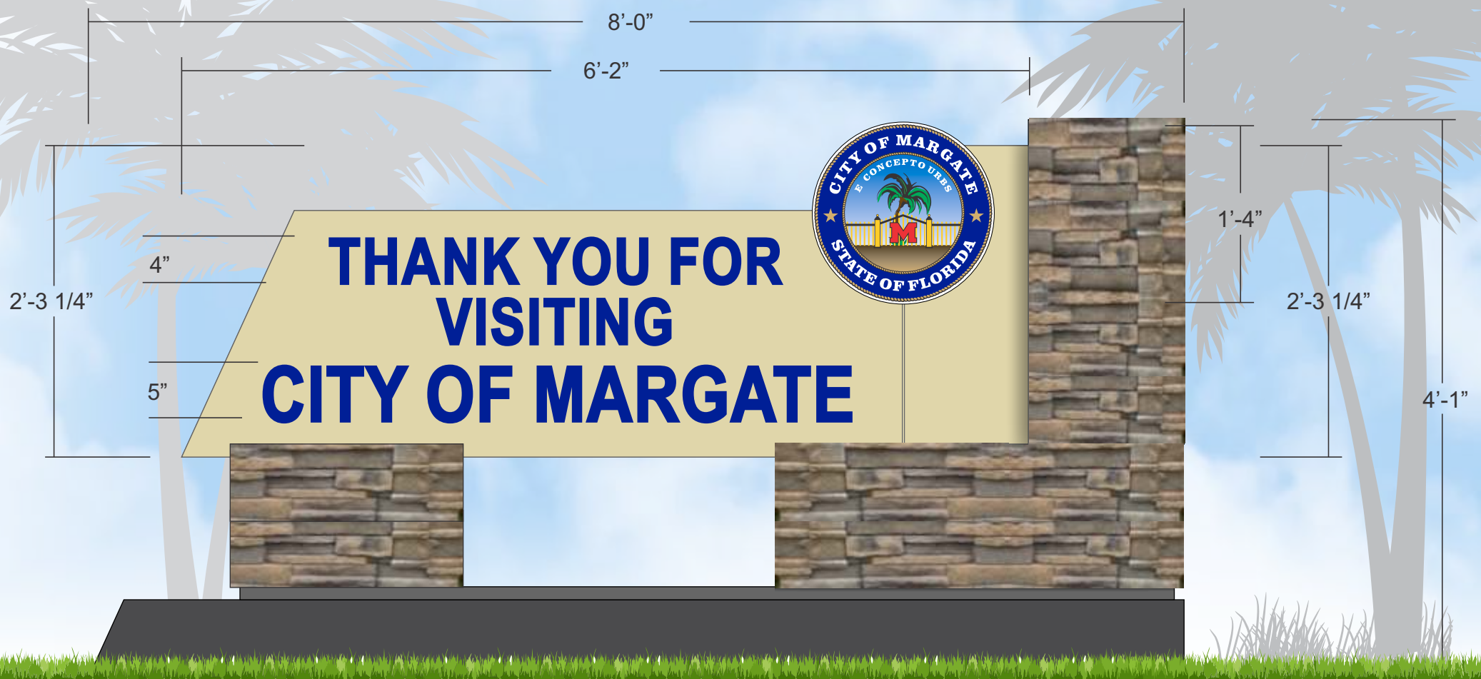
D/F MONUMENT SIGN ELEVATION REAR ELEVATION
