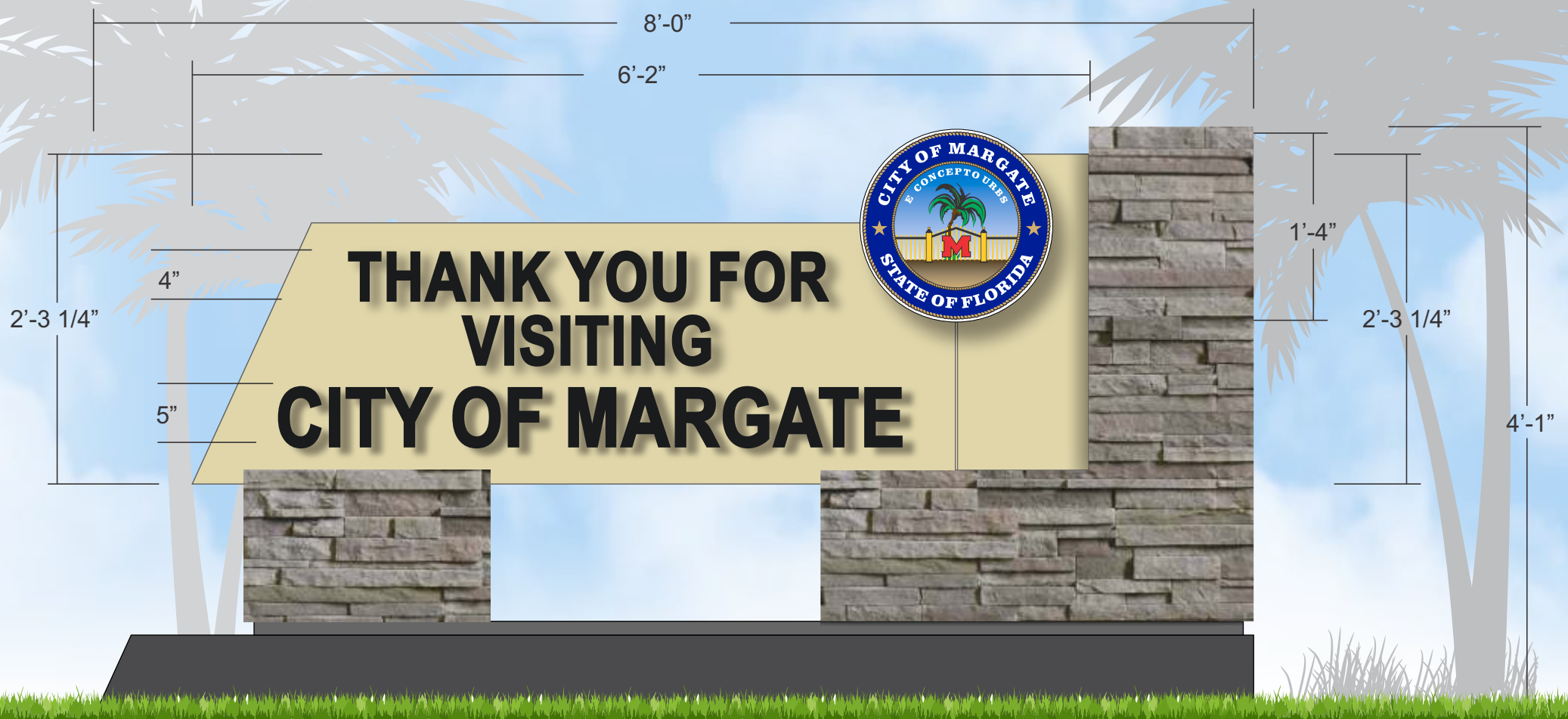
D/F MONUMENT SIGN ELEVATION REAR ELEVATION
