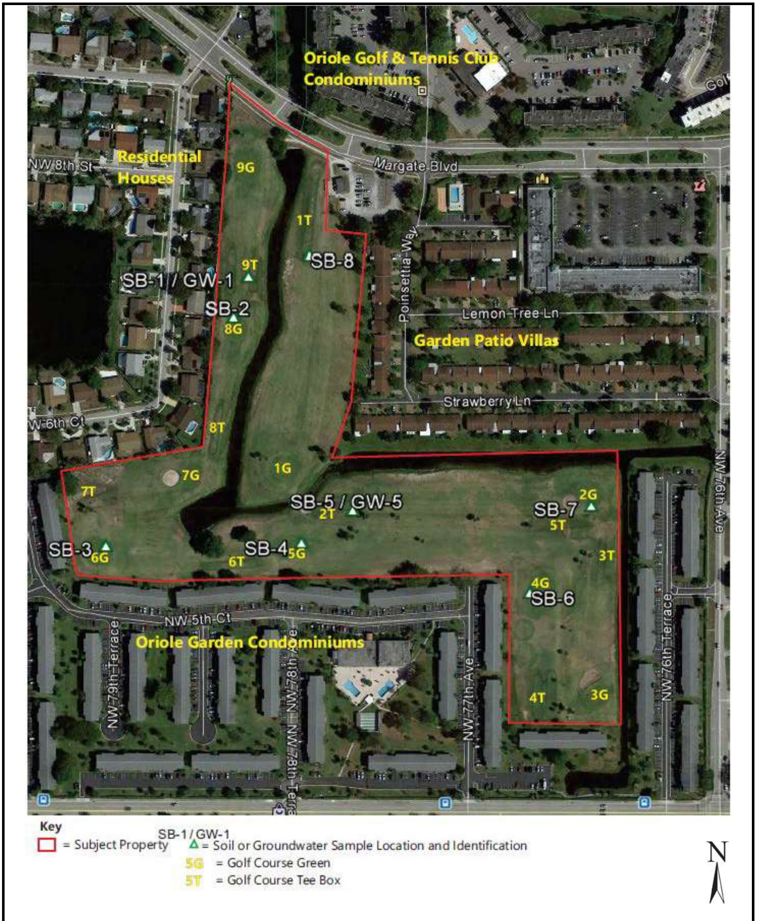
FIGURE 3: SITE PLAN SHOWING SAMPLE LOCATIONS Project No. 18-206246.1
