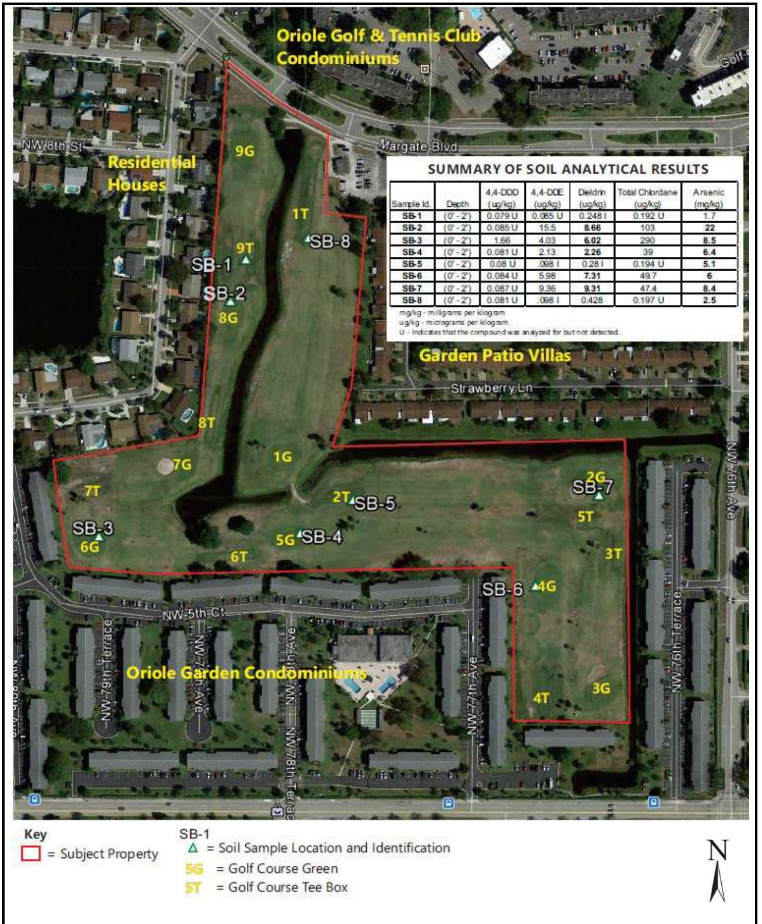
FIGURE 4: SITE PLAN SHOWING SOIL CONCENTRATIONS Project No. 18-206246.1
