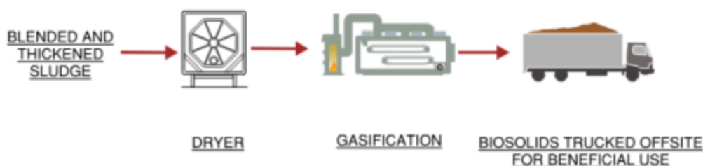
Dryer and Gasification Process Flow Diagram
