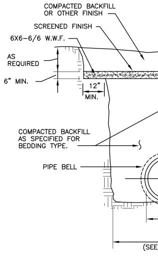
BRACING 12**'** MIN. SHEETING (SEE NOTE 1) PROTECTIVE CONCRETE SLAB SHEETED TRENCH
