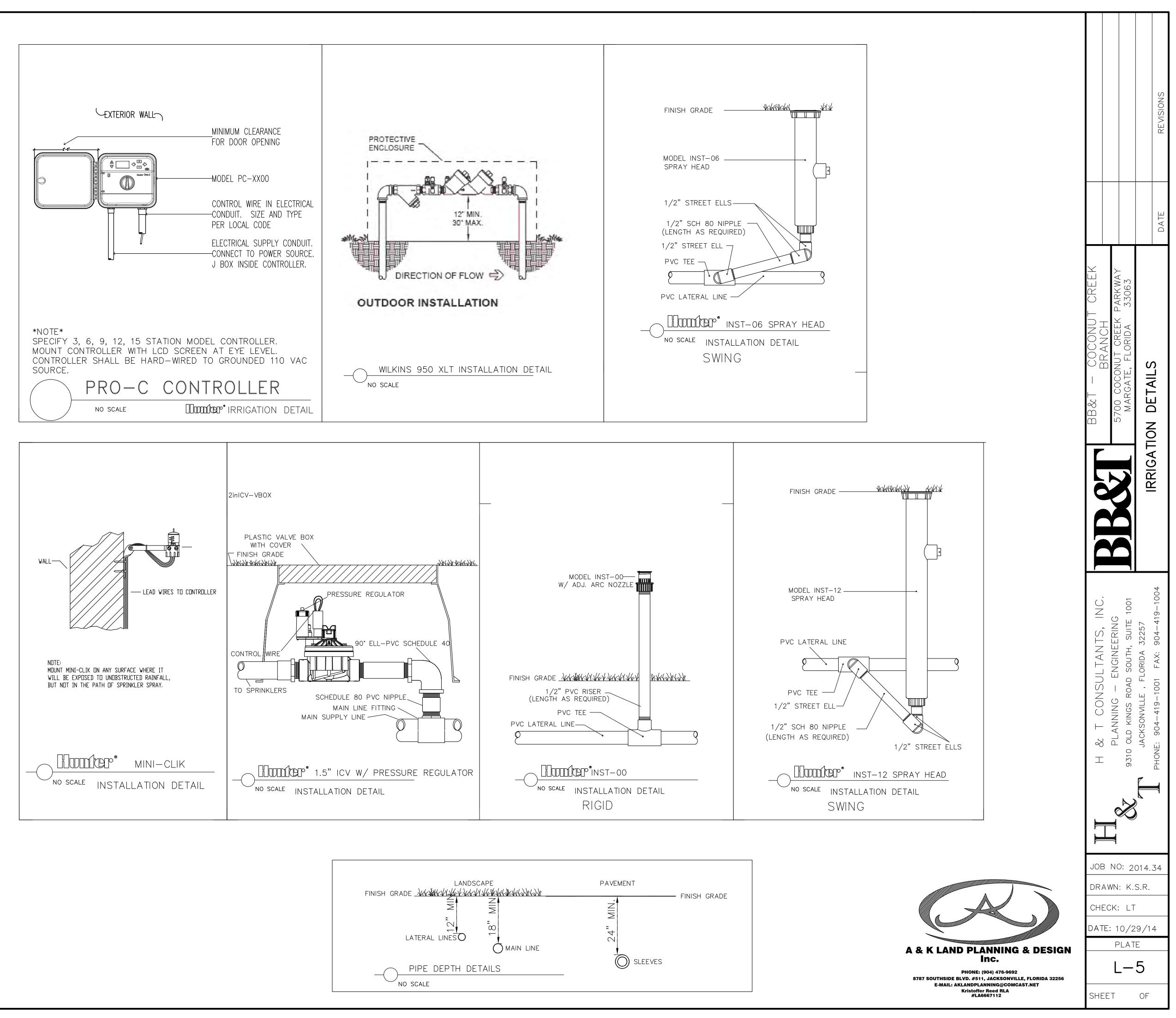
Irrigation Contractor shall be responsible for all applicable fees and permits. All Pipe and Wire under paving shall be placed in Schedule 40 P.V.C. Sleeves for the full pavement coverage length and shall be at least 24" below grade.
