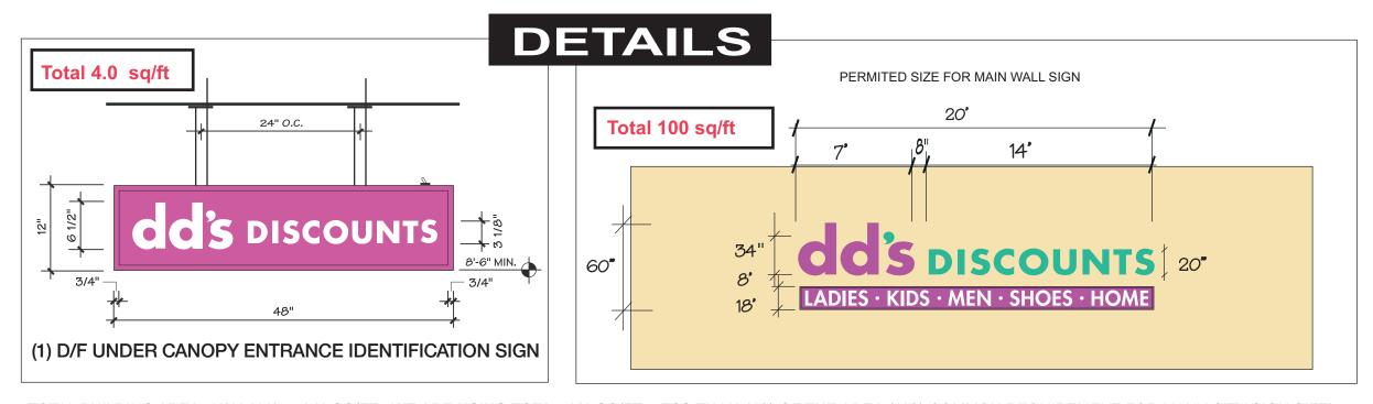
TOTAL BUILDING AREA 42' X 120' 5,040 SQ/FT WE ARE USING TOTAL 440 SQ/FT LESS THAN 10% OF THE AREA (10% COMMON REQUIREMENT FOR MANY CITY SIGN SIZE)
