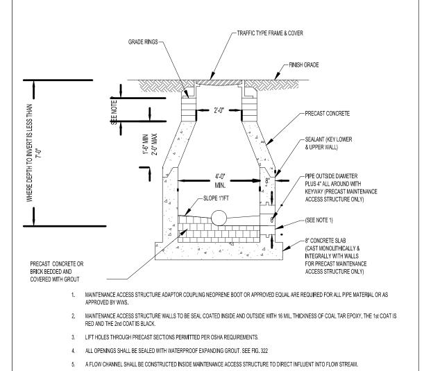
THE CHIMNEY AREA SHALL BE MINIMUM OF 4" AND A MAXIMUM OF 12" IN HEIGHT. A MINIMUM OF 3 GRADE RINGS SHALL BE INSTALLED. SET IN 2 STRIPS OF SEALANT/ADHESIVE COMPOUND ON EACH SEALING FACE.
