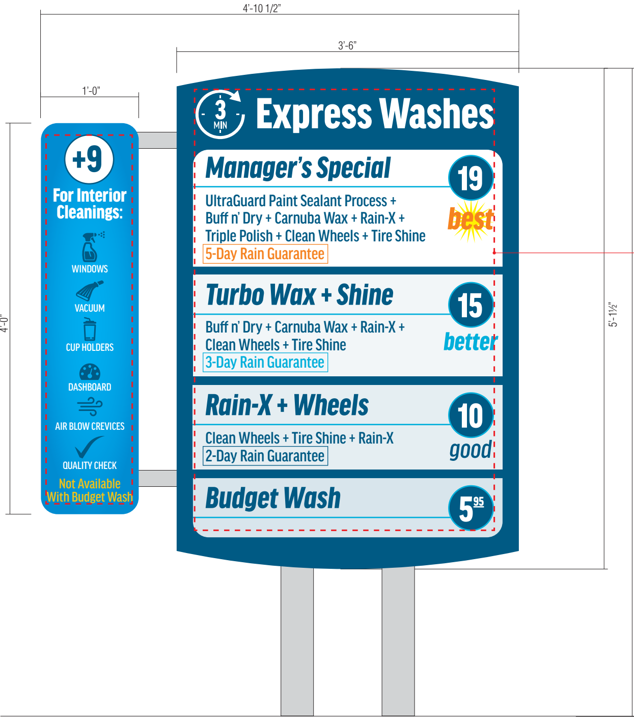
C1 | Scale: 1" = 1'-0" Total Sign Area: 24.98 sq. ft. Total Copy Area: 3.28 sq. ft. + 13.5 sq. ft. = 16.78 sq. ft. (67% of total sign area)
